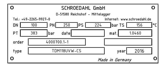
Figure 9 Example of a nameplate of the type TDM
