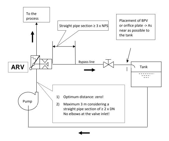
Figure 11 Schematic representation of the installation conditions for the pump protection valve
