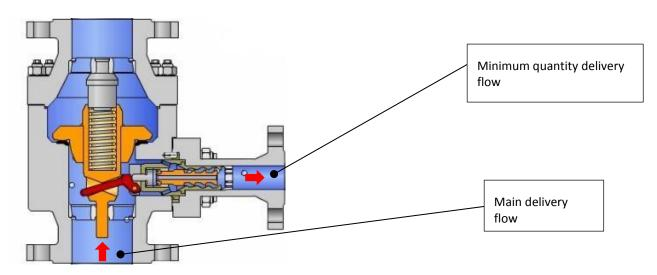
Figure 3 TDM valve with closed non-return plug and open bypass
