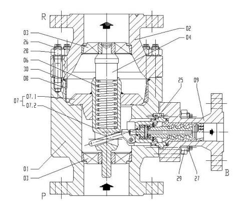
Description Item 01 Lower body 02 Upper body 03 Valve stemguide 04 Guide bolt 06 Spring Non-return plug assembly 07.1 Non-return plug 07.2 Stem 80 Liner or venturi ring 09 Bypass branch 25 Guide Pin 26 Stud bolt 27 Stud bolt 28 Hexagon Nut 29 Hexagon Nut 30 O-ring
